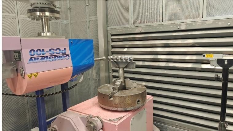
Figure 14. CGS thermal spray system setup with the torch in the rest position between cycles
