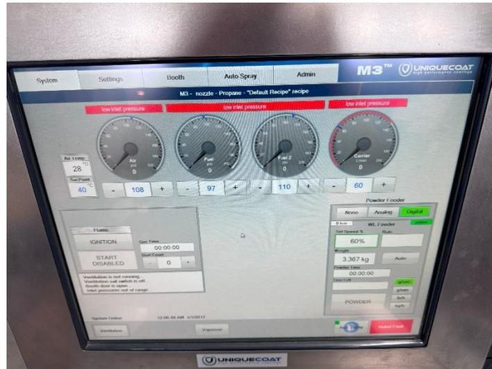
Figure 26. SYSTEM tab - graphical representation of the process parameters of the whole system
