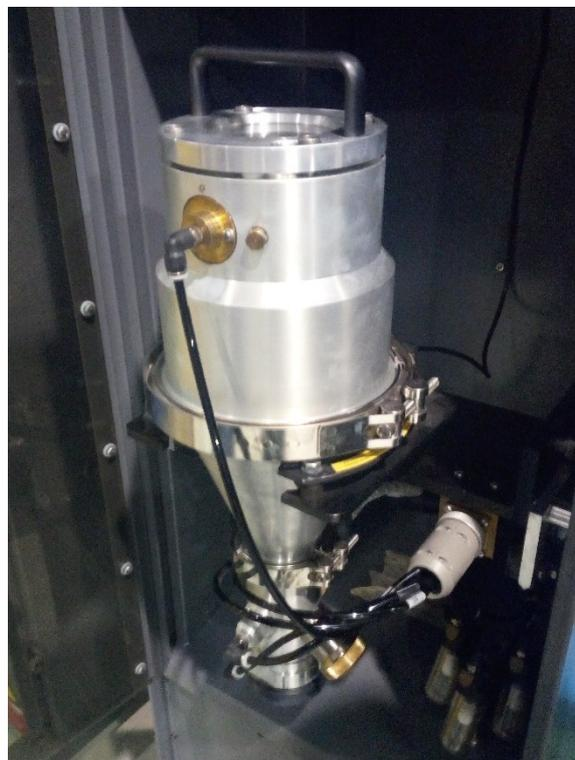
Figure 4. Fluidized-bed pressurized hopper installed onto the load cell in the gravimetric powder feed system
