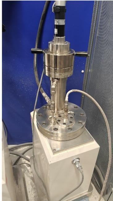
Figure 12. Rotary pressurized powder feed system
