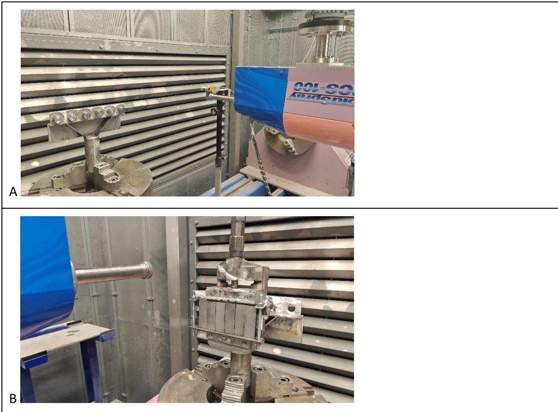
Figure 11. Sample holder design mounted for (a) cylinders only, and (b) plates only.
