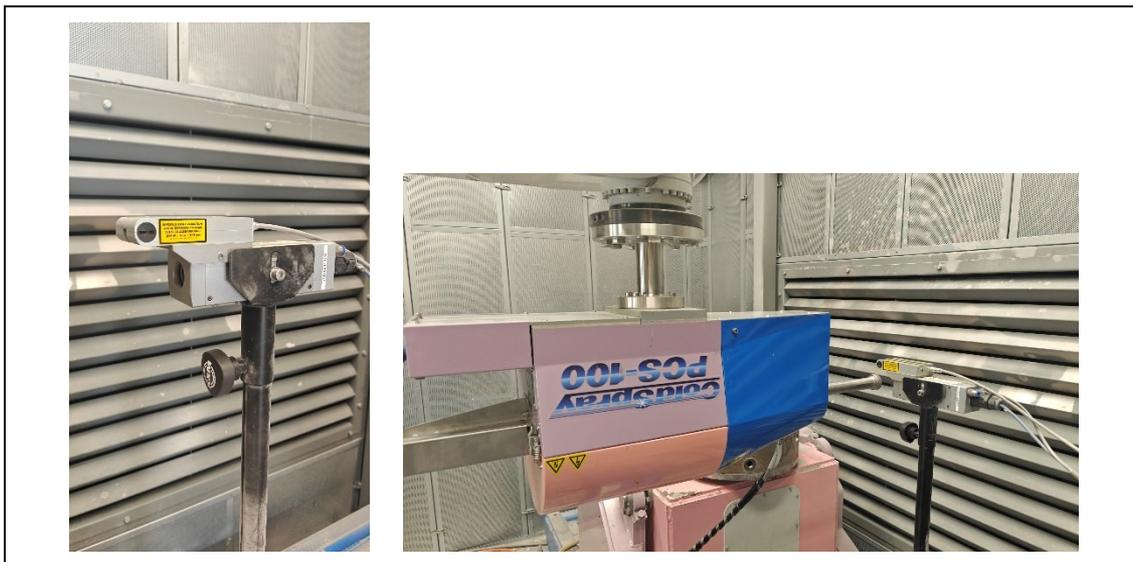
Figure 13. TITOMIC Hiwatch 2 system and PCS100 allocation for velocity measurements
